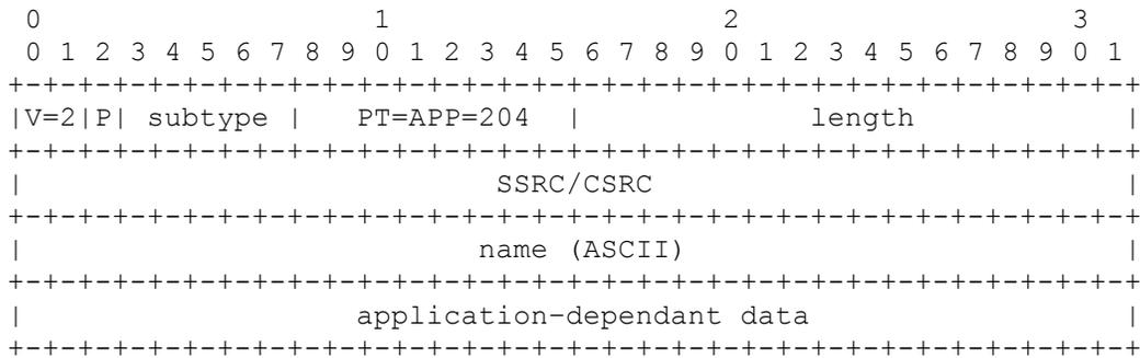
**Figure 3: RTCP APP Packet Structure for Use in this TR**
