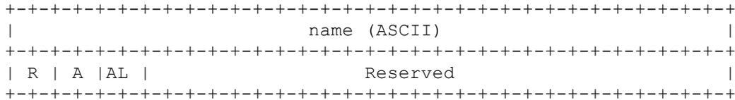
**Figure 4: Application-dependant Data Field Parameters for Sender RTCP APP Packet Structure**
