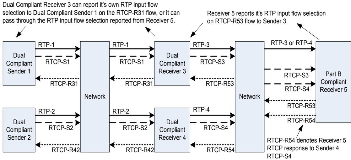
**Figure 6: Example System for Dual Compliant Devices**
