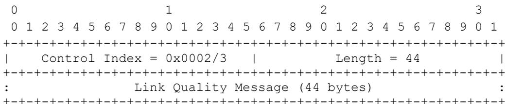
Figure 5: Link Quality Message encapsulation in Advanced Profile
