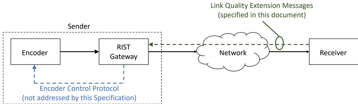
Figure 1: System Architecture
